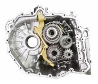
The DSG 6 gearbox is an automatic Volkswagen AG gearbox. DSG stands for 'Direktschaltgetriebe' or 'Direct Shift Gearbox' and the 6 stands for six forward gears. The designation 'DQ250' is also used for this gearbox. The Q ('Quermotor') indicates that this gearbox is used for transverse engines.
