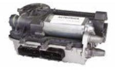
The most vulnerable part of the Durashift is the clutch actuator. It is mounted in a plastic housing and can quickly start leaking. If you suspect that the clutch actuator is leaking, carry out the official bleeding procedure at all times (see at page 124). The clutch actuator will certainly leak if it is defective.
