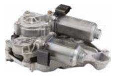
The gear selector is still controlled in the "old-fashioned" way by the TCU. This means that CAN messages are not used, but power, ground and signals for direction and time are used. Because both signals are necessary to activate these "smart" electric motors, it is unfortunately not possible to connect power and ground to test the electric motors yourself.
