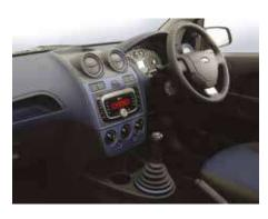
The Durashift system is a so-called robotised manual gearbox based on Ford's iB5 five-speed manual gearbox. The Durashift gearbox allows both automatic shifting and shifting with the selector lever. In both cases, the clutch is operated automatically.
