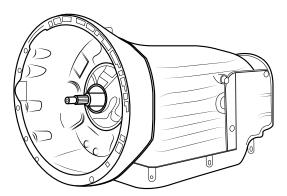
The 7G-Tronic was introduced on 5 different Mercedes-Benz models with V8: E500, S430, S500, CL500 and SL500. The gearbox was subsequently also used on certain 6-cylinder diesels such as, for example, cars with the 320 CDI engine. However, the cars with V12 engines (S600, S65 AMG) carried on using the older 5G-Tronic, because this gearbox could handle a torque up to 1079 Nm. The 7G-Tronic
