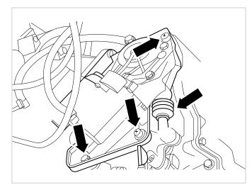
2. Disconnect both plugs from the shift actuator: the black plug is on top of a shift motor, the grey plug is blocked on the side of a shift motor. See illustrations above.
