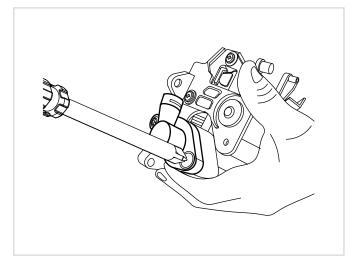
5. Remove the clutch pump screws.
