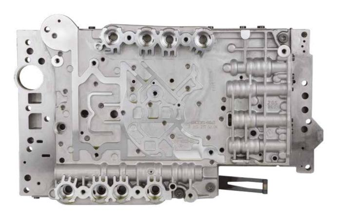
The valve body: a labyrinth of fluid lines, consisting of 2 metal housings and a dividing plate.
