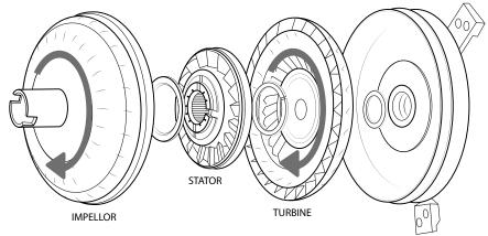
Exploded view torque converter.
