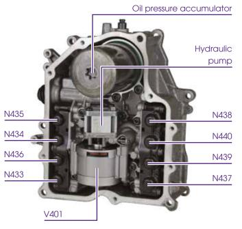
system pressure in the control unit remains between 40 and 60 bar.
