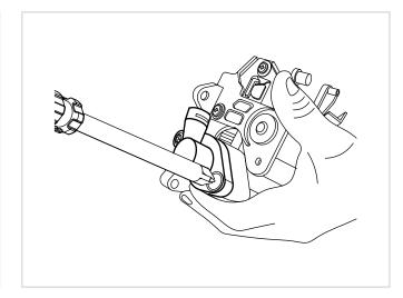
5. Remove the clutch pump screws.
