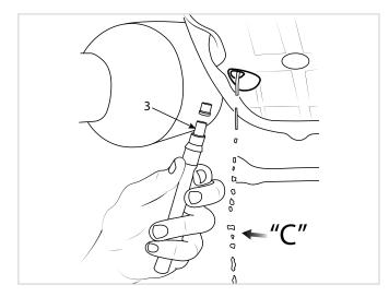
13. Remove the adapter "2". Excess oil now starts owing out of the sump.
