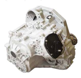
The DSG 7 gearbox is an automatic double clutch gearbox. DSG stands for "Direktschaltgetriebe" or "Direct Shift Gearbox" and the 7 indicates that there are seven forward gears. For this gearbox the designation 'DQ200' is also used. The Q ('Quermotor') indicates that this gearbox is used for transverse engines.
