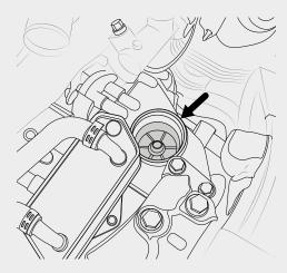
If the contamination of the oil becomes so great that the gearbox oil filter becomes clogged, the oil will circulate through the bypass, which means that the oil will no longer be filtered. Wear and tear can then accumulate on the sensors and in the shift and control valves, causing the Mechatronic to malfunction and adversely affecting the operation of the gearbox. It is therefore important that the oil and filter of the DSG 6 gearbox are changed every 60,000 km.
