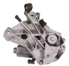
Real differences should be sought more in the assembly of the components. Ford has applied the Mechatronic to a gearbox of its own and therefore the mounting position differs from that of Opel. The wiring has also been modified slightly: whereas Opel always uses a standard wiring harness, Ford has some variations.
