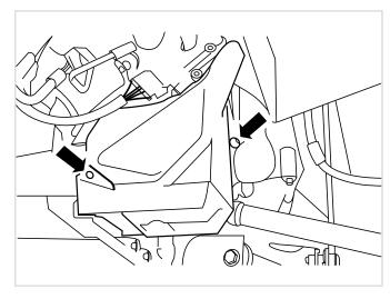
3. Attach both plugs to the shift actuator: the black plug belongs on top of a shift motor, the grey plug belongs on the side of a shift motor. See illustrations above.
