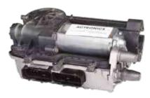
The most vulnerable part of the Durashift is the clutch actuator. It is mounted in a plastic housing and can quickly start leaking. If you suspect that the clutch actuator is leaking, carry out the official bleeding procedure at all times (see at page 124). The clutch actuator will certainly leak if it is defective.
